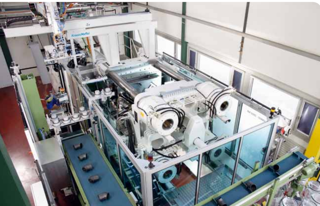
Manufacturing cell with industrial robot to produce pipe connecting fittings, integrated customer packaging system
