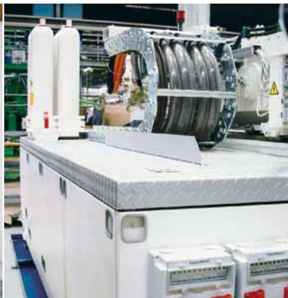
Encapsulated hydraulic drive, soundproof housing
