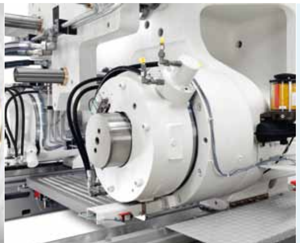
Locking element and clamp force cylinder for very fast machine movements
