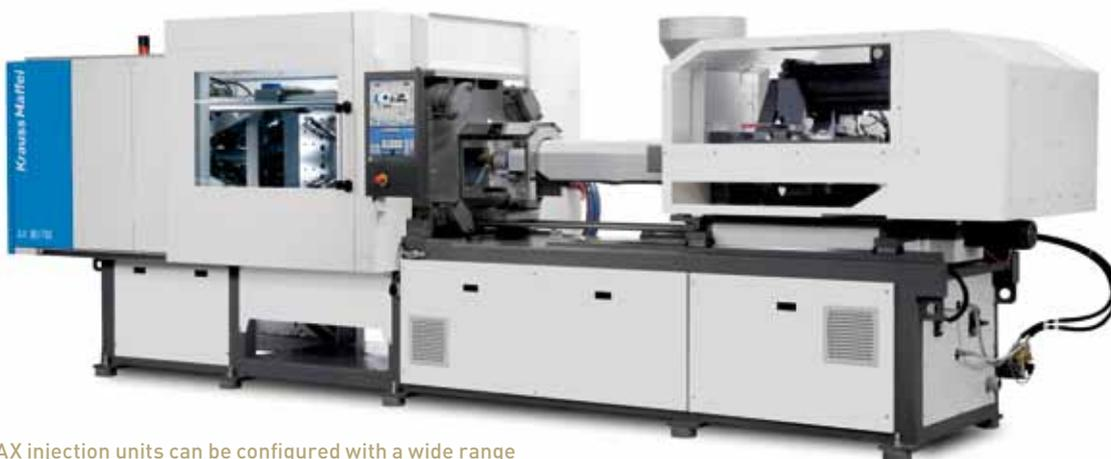
AX injection units can be configured with a wide range of plasticizing systems – interchangeable with those of our EX and CX series.
