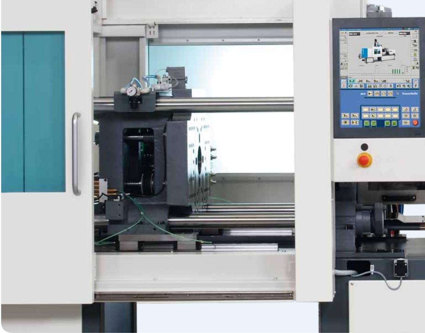
Large double precision linear guides for the moving platen guarantee absolutely repeatable mold closing.
