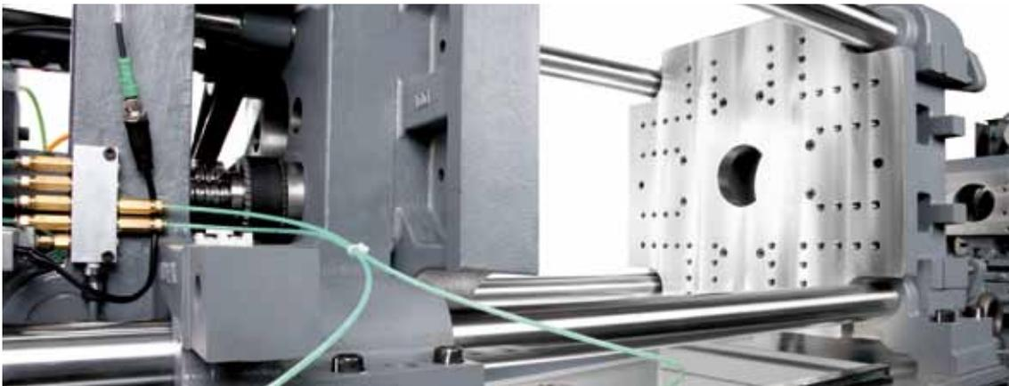
The solid “box” construction of the mold fixing platen ensures even application of force. The generously dimensioned guide system contributes to excellent platen parallelism.
