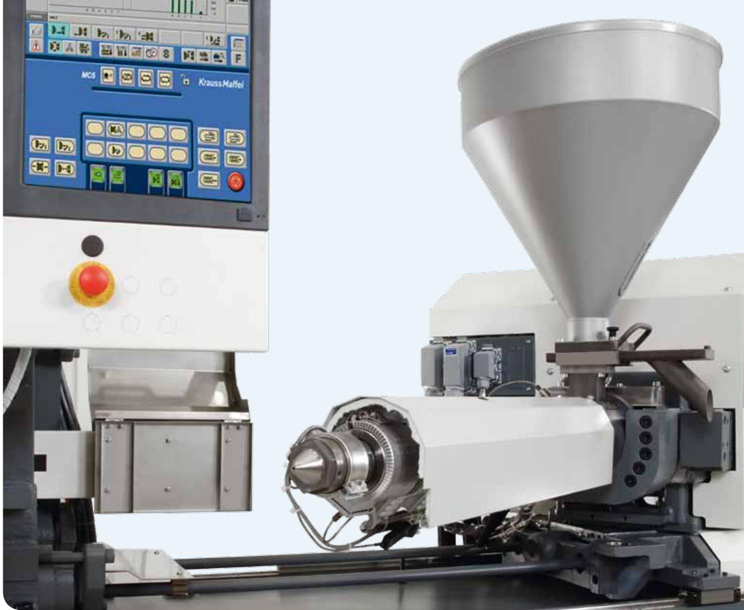
A swing-out plasticizing unit and nozzle viewing flap make it easier to monitor and maintain all key components of AX machines.
