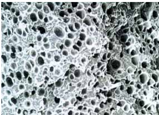
Cross-section through an injection molded part made by the MuCell® process. The foamed center and the compact outer skin form a unit. This type of structure produced by physical foaming is also called integral foam.
