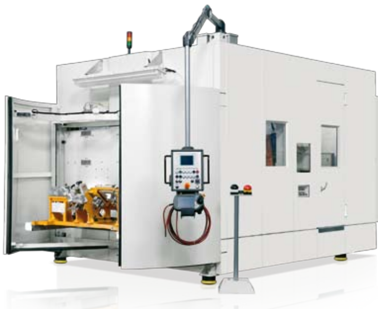
KraussMaffei's Routing Star is an automated cutting cell for flexible production
