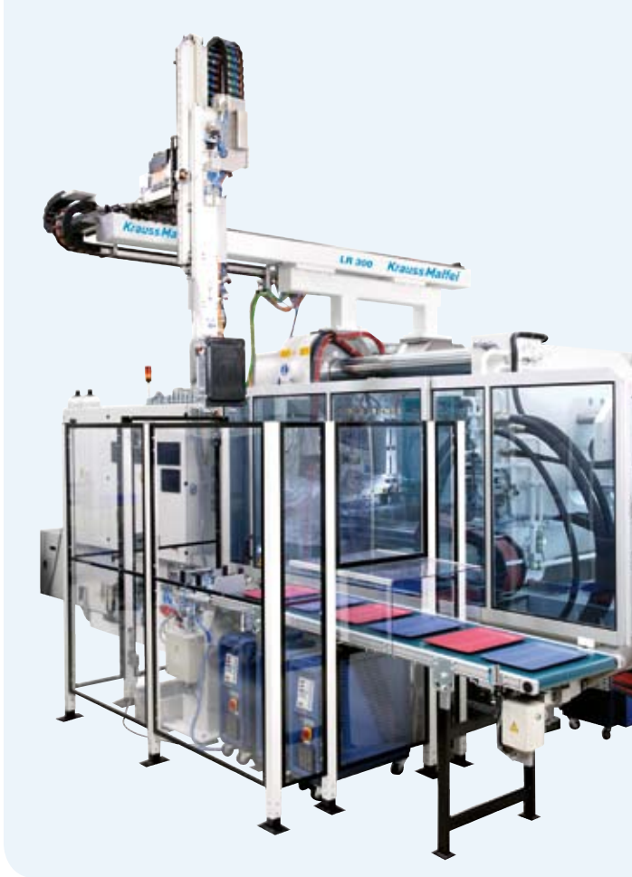
Integrated LR 300 linear robot in a manufacturing cell for a SkinForm® tray
