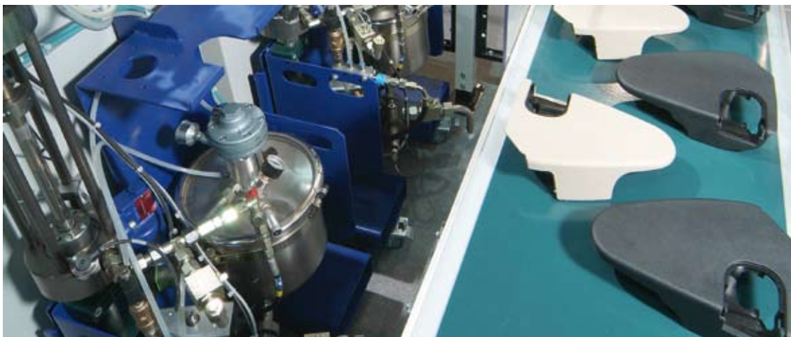
Colour change from shot-to-shot with the flexible MicroDos colour management system demonstrates the true performance of the mixing head in this SkinForm® application
