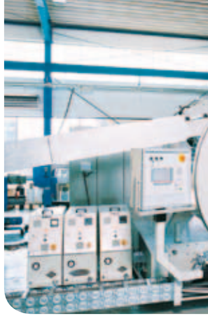
PlanetCalander – flexible polishing stack for producing optical-grade sheet
