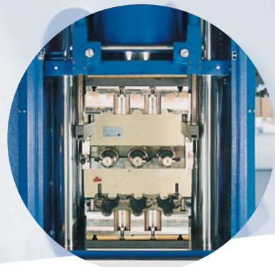
hydraulic ejectors in 4-fold synchronized execution
