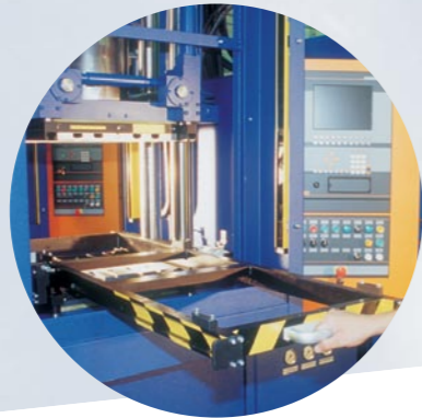
frame style center plate shuttle, manually or hydraulic operated
